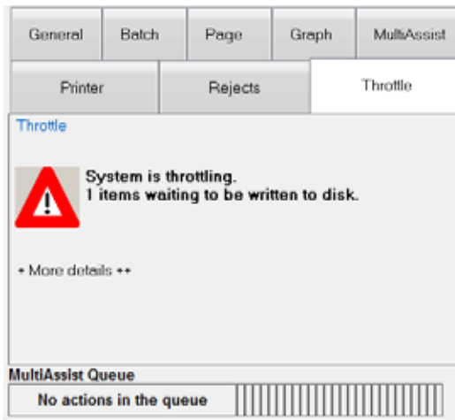
Figure 9: The system in a throttling state - detail of the runscreen
